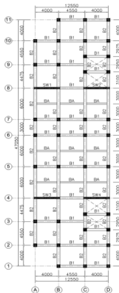
Fig. 1. Typical plan layout of a twelve-story building considered
