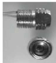
Fig. 3. Optically immersed LED MID IR sensor
