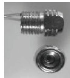
Fig. 3. Optically immersed LED MID IR sensor
