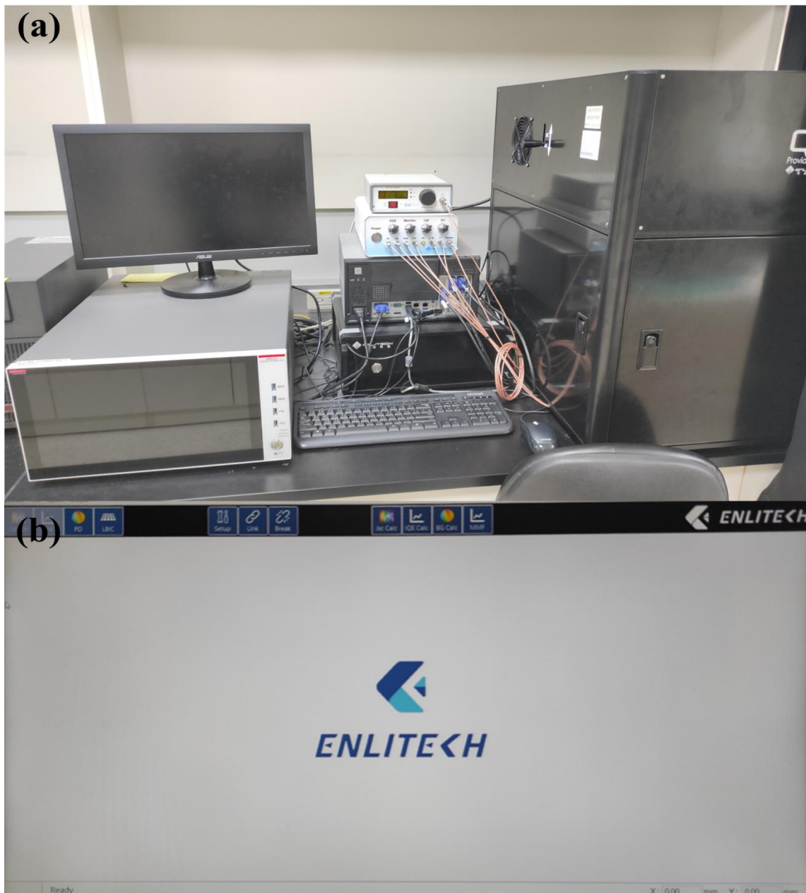
Figure 3.7 (a) QE-R system and (b) software for EQE and responsivity measurement.
