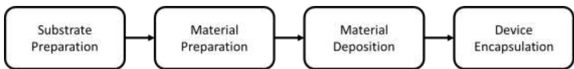
Figure 3.8 Device fabrication process for the OLEDs device.
