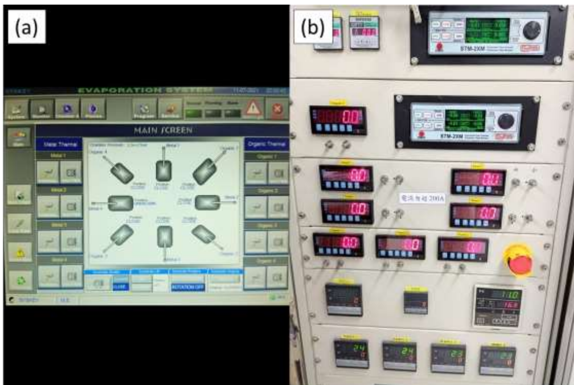
Figure 3.14 Computer system in thermal evaporation system (a) and current controller and temperature sensor display (b).
