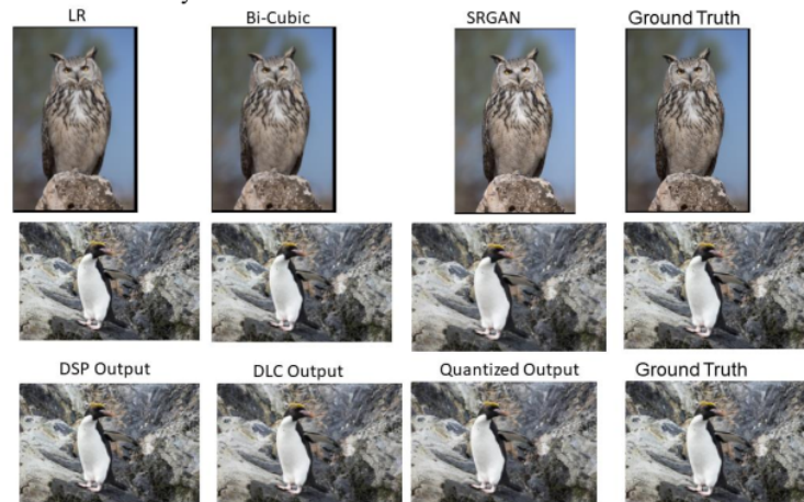
Figure 4. LR Images, Generated HR Images of Bi-Cubic and SRGAN Model, and Ground Truth Images and SRGAN output on DSP with Quantized and Non-quantized Images
