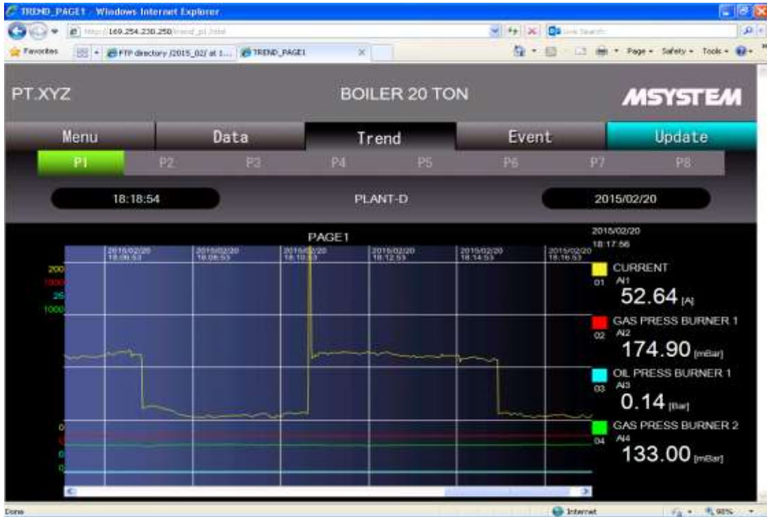
Fig. 11. Overview of Trend Display for Four Parameters (Analog Input).
