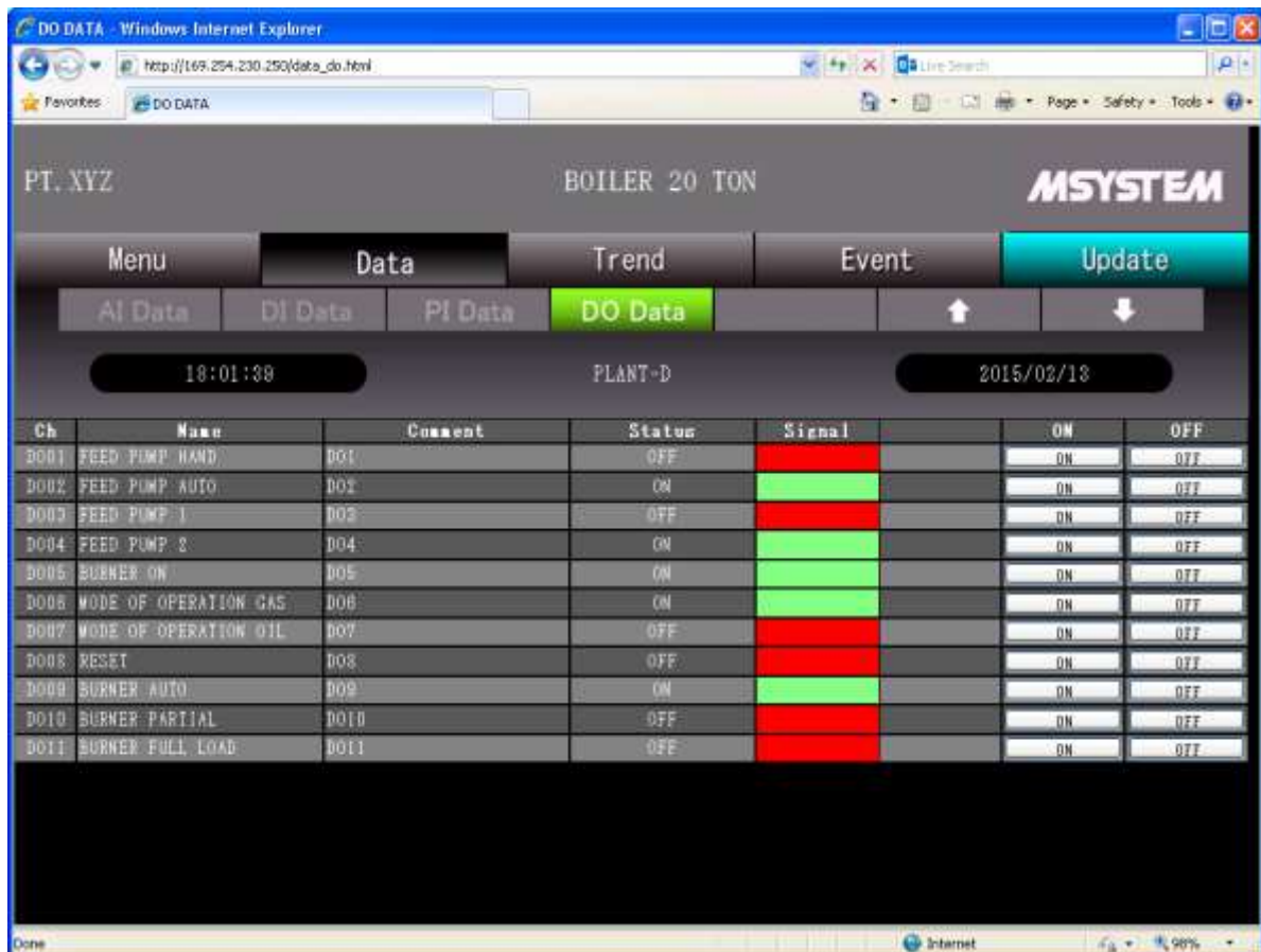
Fig. 8. Overview of PC Display for Remote Access Control (Digital Input).
