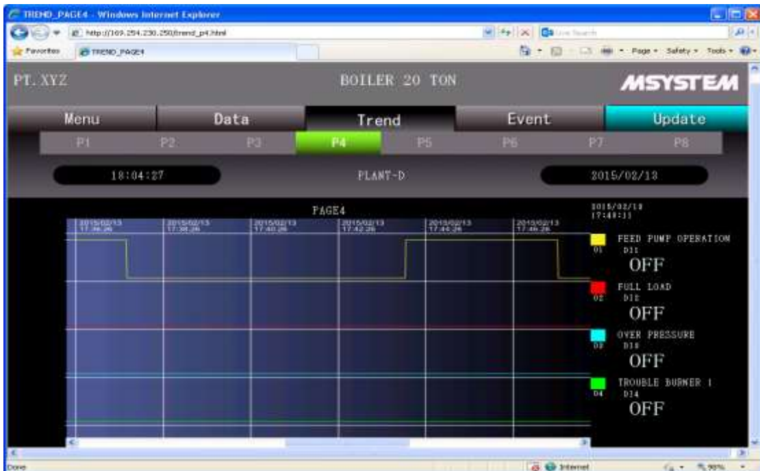
Fig. 12. Overview of Trend Display for Four Operational Statuses (Analog Input).
