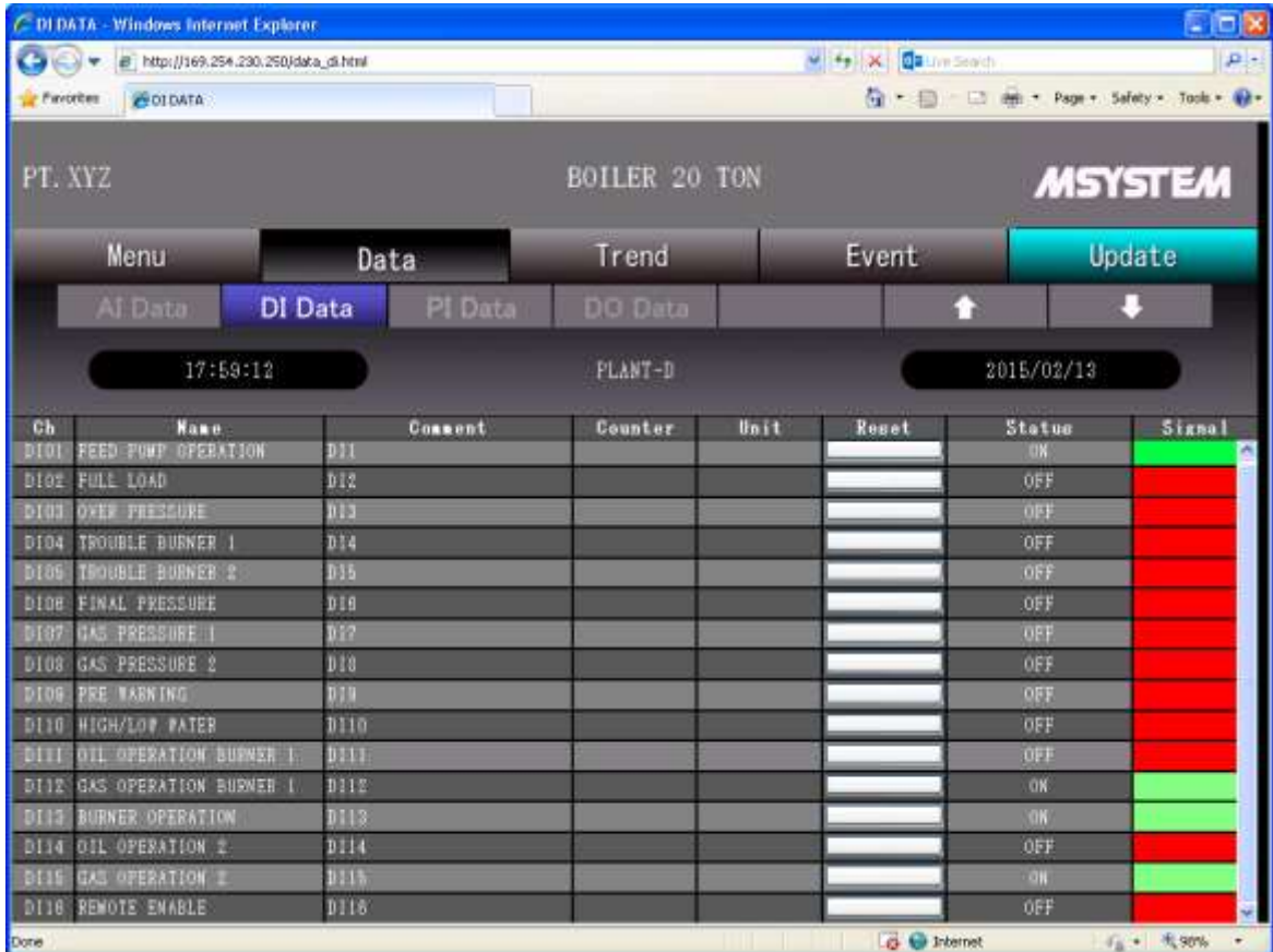
Fig. 9. Overview of PC Display for Remote Access Control (Digital Input).
